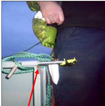
Securing pin for bulwark door protruding from its socket
