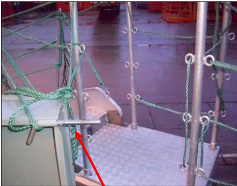
Securing pin for bulwark door protruding from its socket
