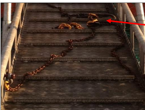
Lifting bridle left hanging over the guard ropes
