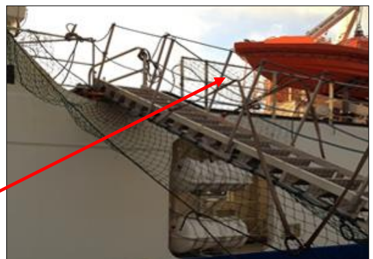
Potential trip hazard from lifting bridle
